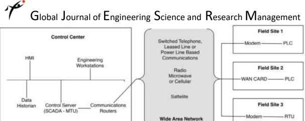
Fig 1: Generic SCADA hardware architecture (Source: NIST SP 800-82)
